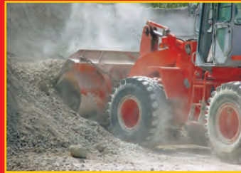
Recycling, crushing and grading concrete for reuse at the Kumeu plant
