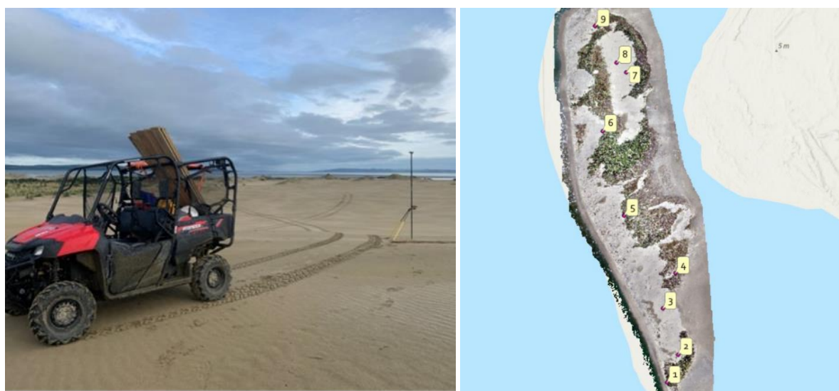
Figure 2-2: Interpine have fixed the location of nine ground control points on Manukapua Island. [Credit Left: Susana Gonzalez (Interpine Group), Right: 0.25 m Aerial photo].
